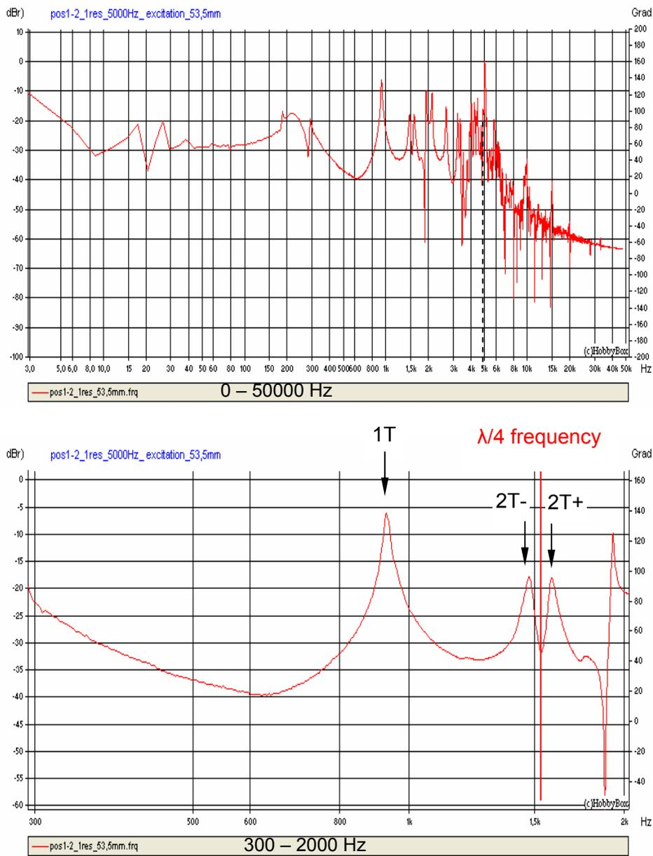
**Figure 3.4.7:** Frequency response, position 1-2, one resonator,  $L/R = 0,49$
