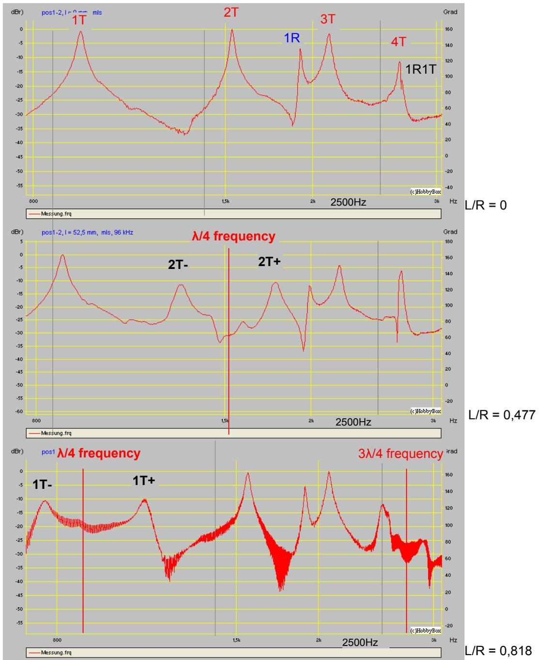
**Figure 3.3.3:** Frequency distribution between 800 and 3000 Hz,  $L/R = 0/ 0.477/ 0.818$  , position 1-2, 42 resonators
