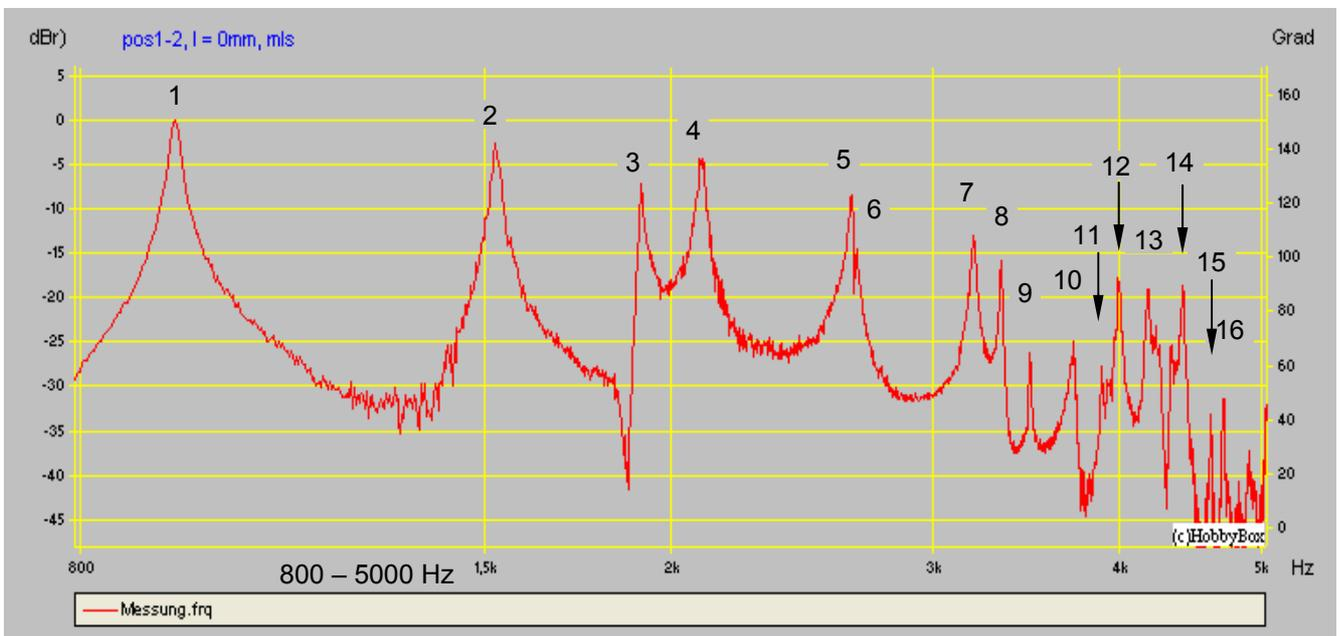
**Figure 3.1.1:** Pulse response and frequency distribution after MLS excitation, position 1-2, mode identification: table 3.1.1
