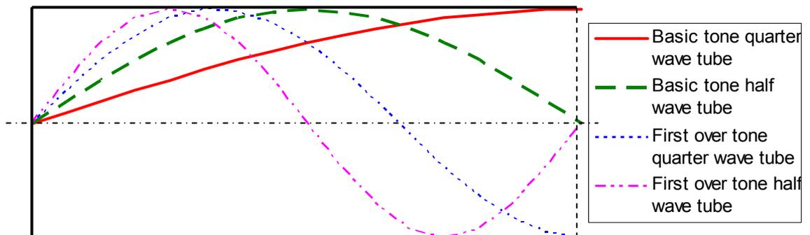
Figure 1.2.1: Velocity distribution in lambda-quarter and lambda-half tubes
