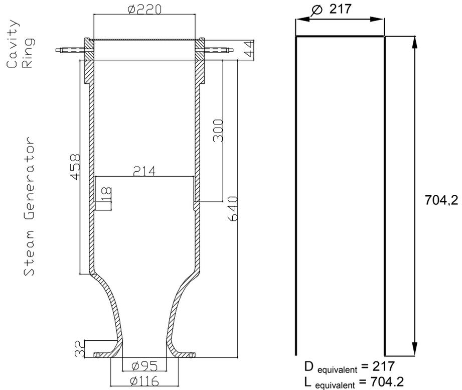
**Figure 2.1.1:** Geometry of steam generator, and equivalent cylindrical geometry assuming the steam generator being a lambda-quarter tube
