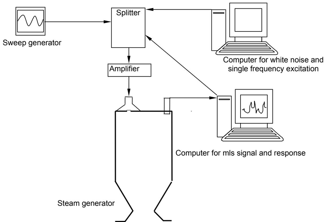
**Figure 2.1.7:** Scheme of signal flow
