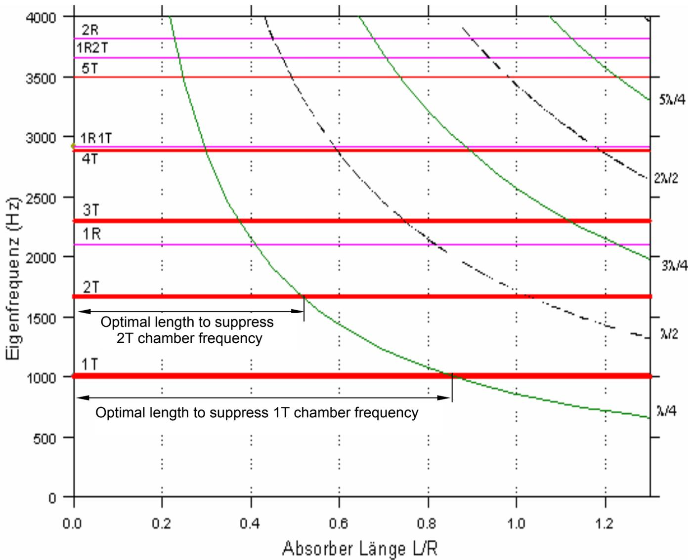
**Figure 1.5.3:** Fundamental chamber frequencies and cavity eigenfrequencies
