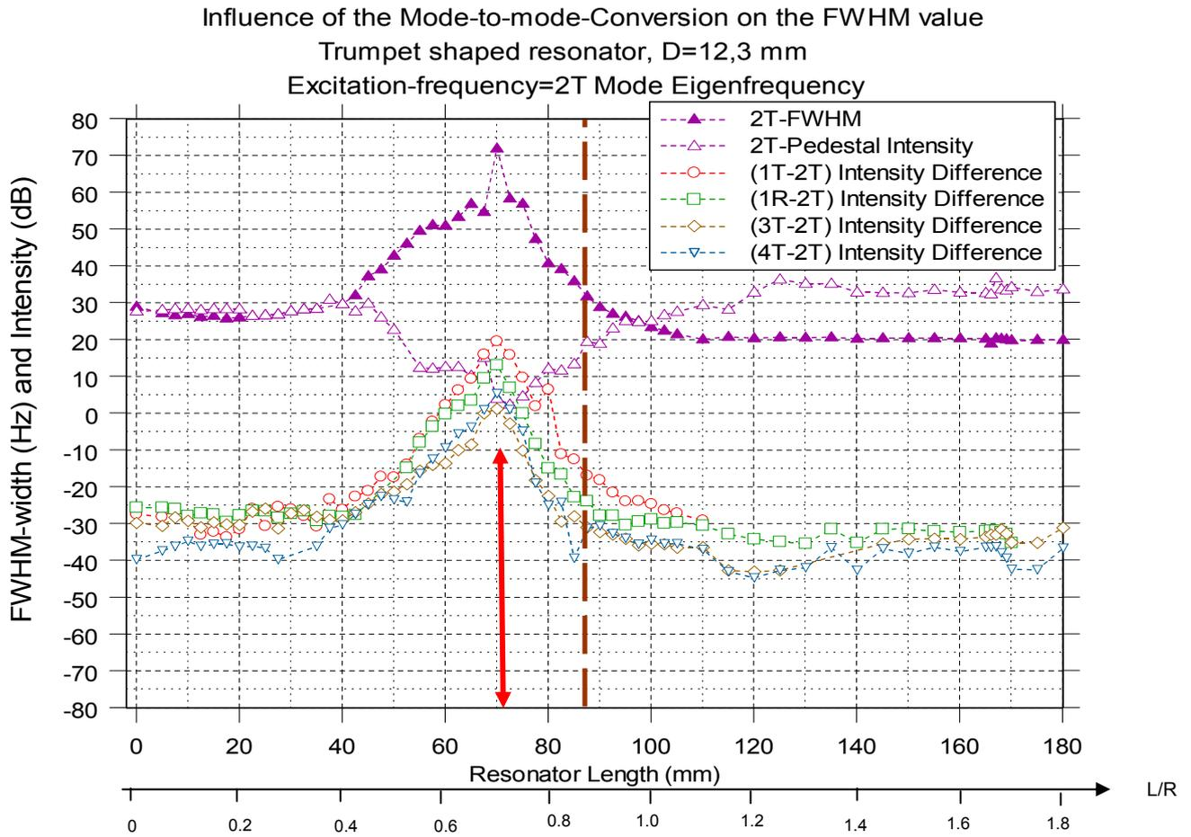
**Figure 1.5.6:** Mode to mode conversion in a cavity ring coupled with one resonator [5]
