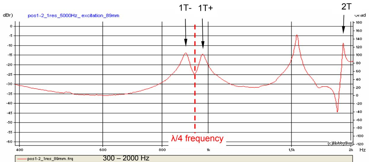
**Figure 3.4.2:** Frequency response, position 1-2, one resonator at  $L/R = 0,809$
