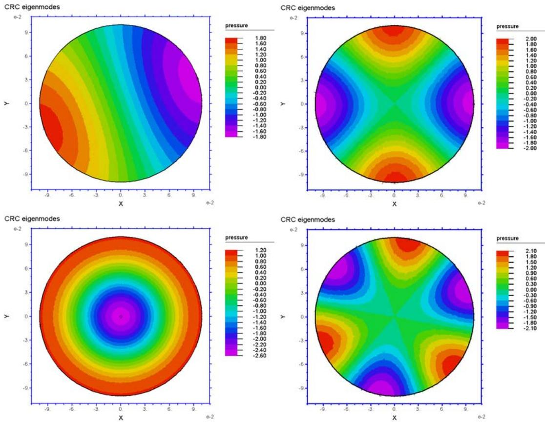
Figure 1.1.1: Pressure distribution in the chamber for the acoustical modes 1T, 2T (top), 1R and 3T (bottom) [8]
