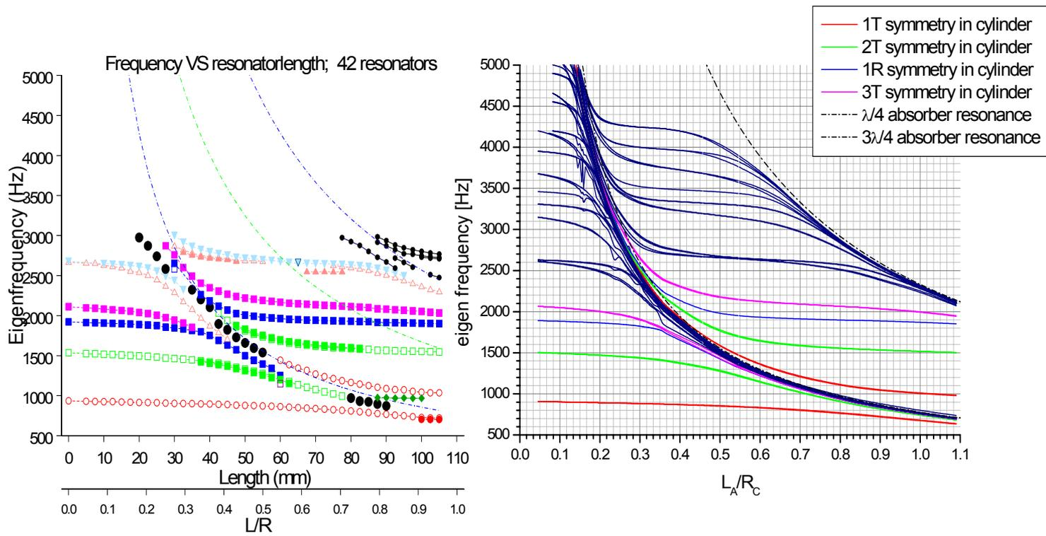
**Figure 3.3.6:** Classification of modes according to calculation of FlexPDE [8], measurement compared with calculus, position 1-2, [2]
