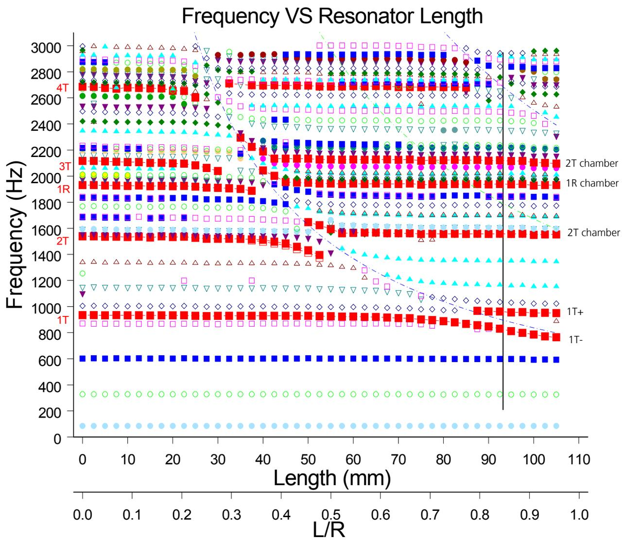
**Figure 3.3.17:** Classification of modes, transverse modes highlighted
