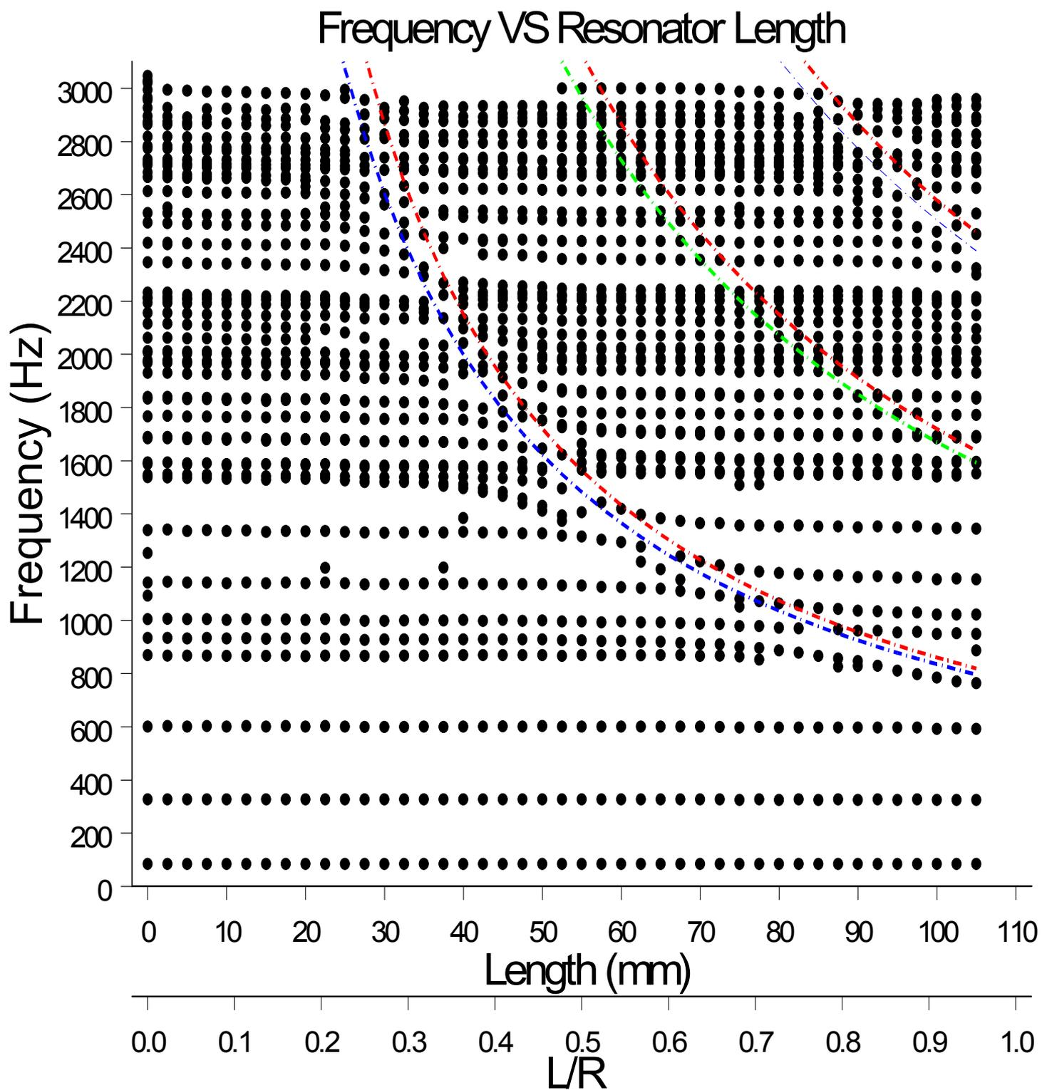
**Figure 3.3.16:** Measured curve of modes, position 1-7, 42 resonators
