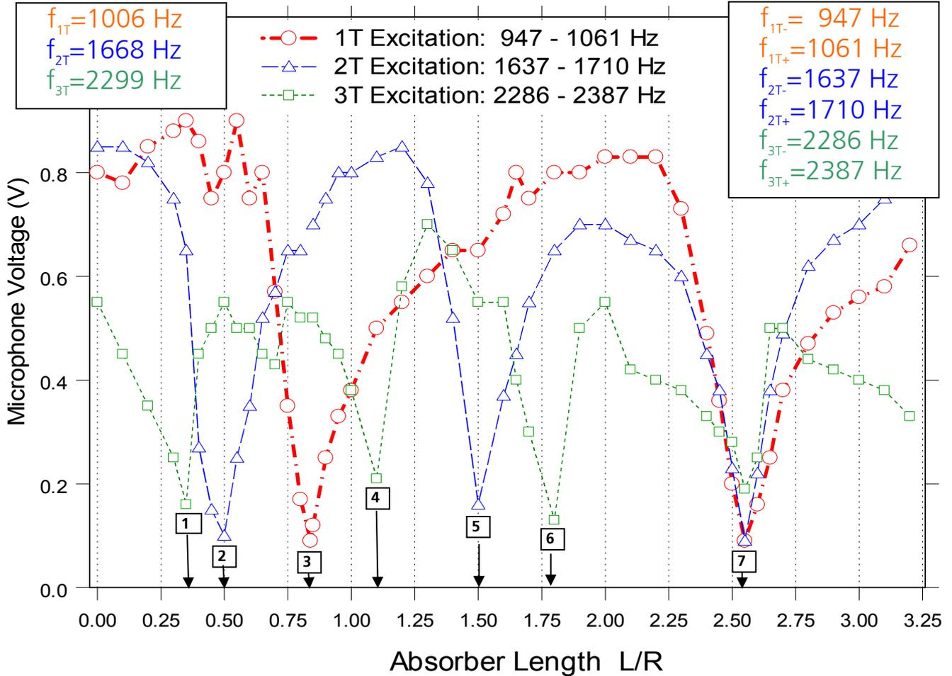
**Figure 4.1:** Microphone signal VERSUS resonator length for a cylindrical chamber coupled with one resonator [12]; excitation with sweeping frequencies in the ranges of  $f_{1T-} - f_{1T+}$ ,  $f_{2T-} - f_{2T+}$  and  $f_{3T-} - f_{3T+}$
