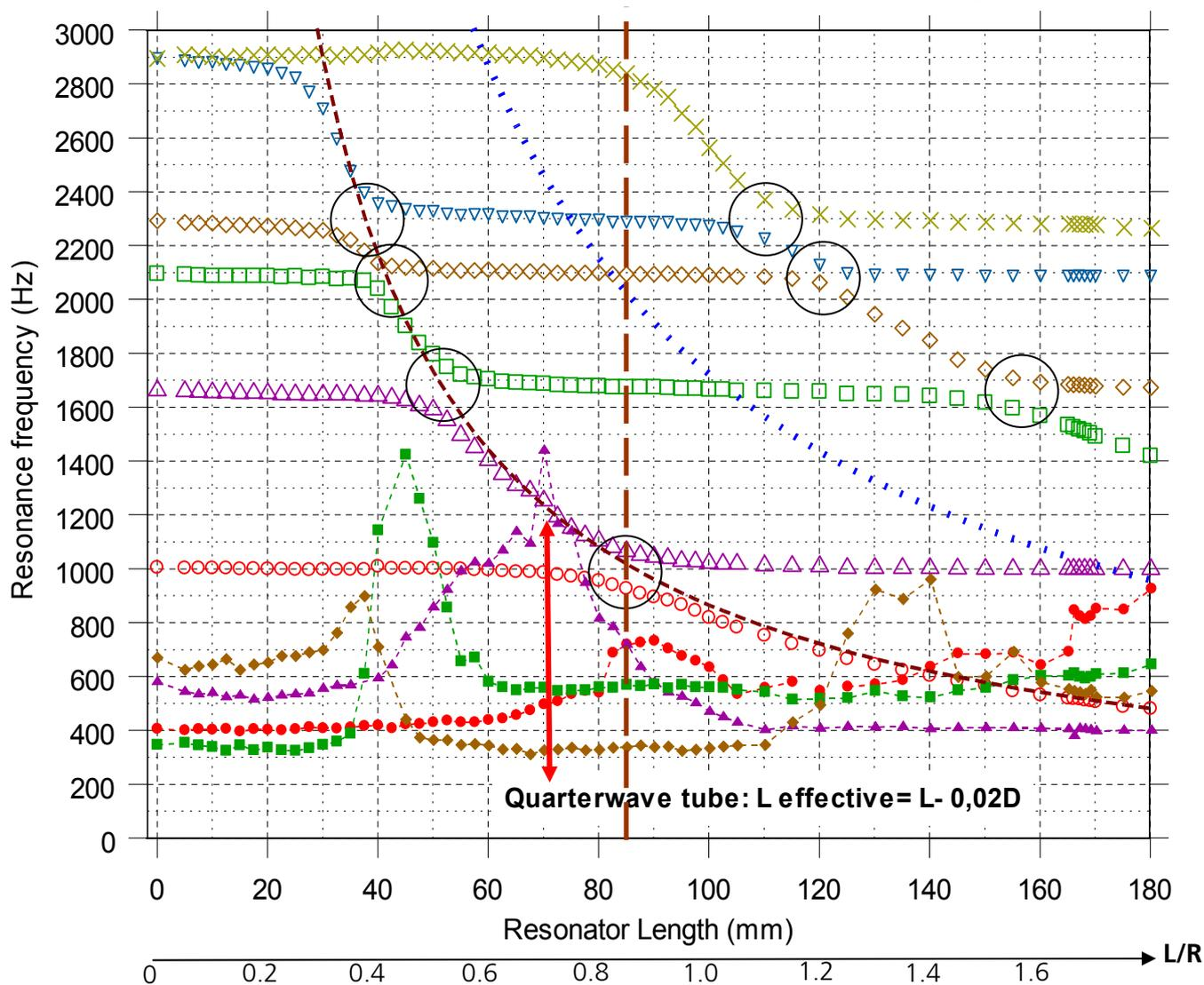
**Figure 1.5.2:** Frequency and FWHM of acoustical eigenmodes in system of CRC coupled with resonator cavity, CRC radius 100 mm [5]
