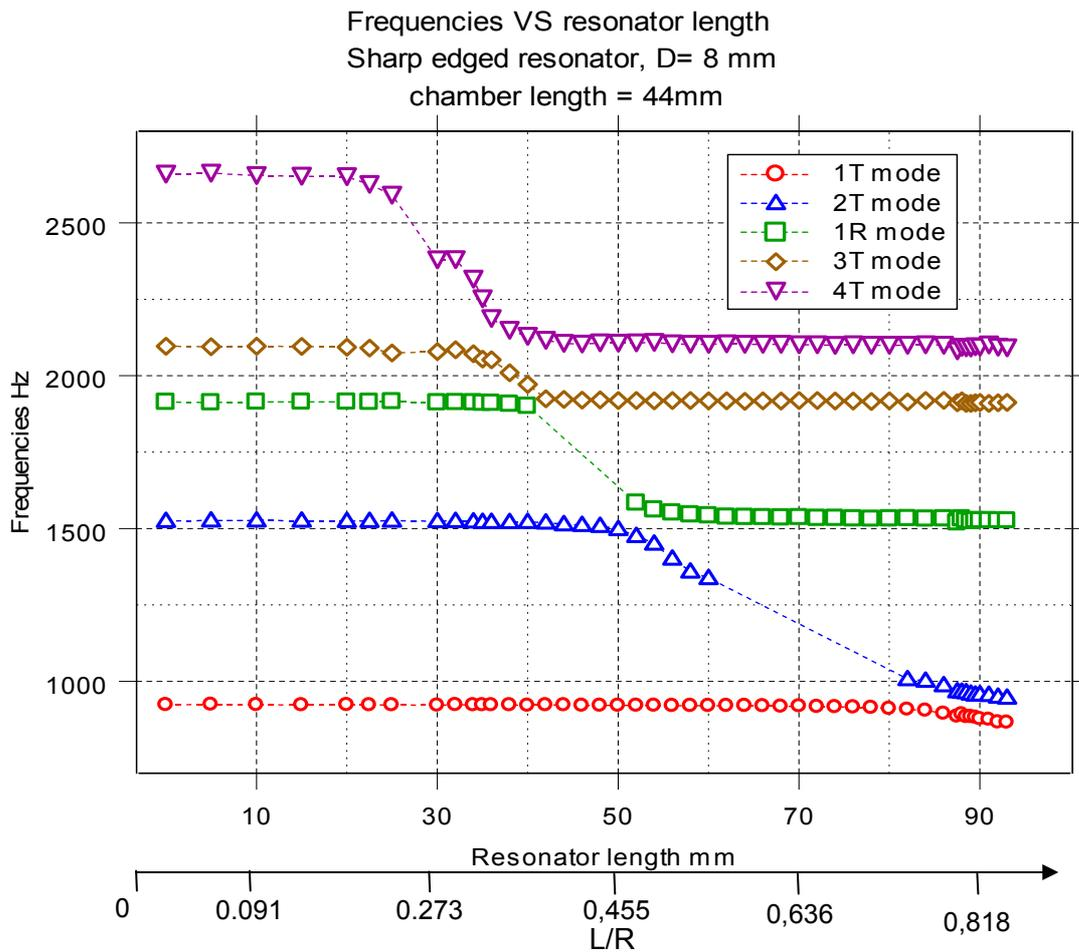
**Figure 3.3.5:** Measured course of the modes for one resonator, position 1-2, [6]
