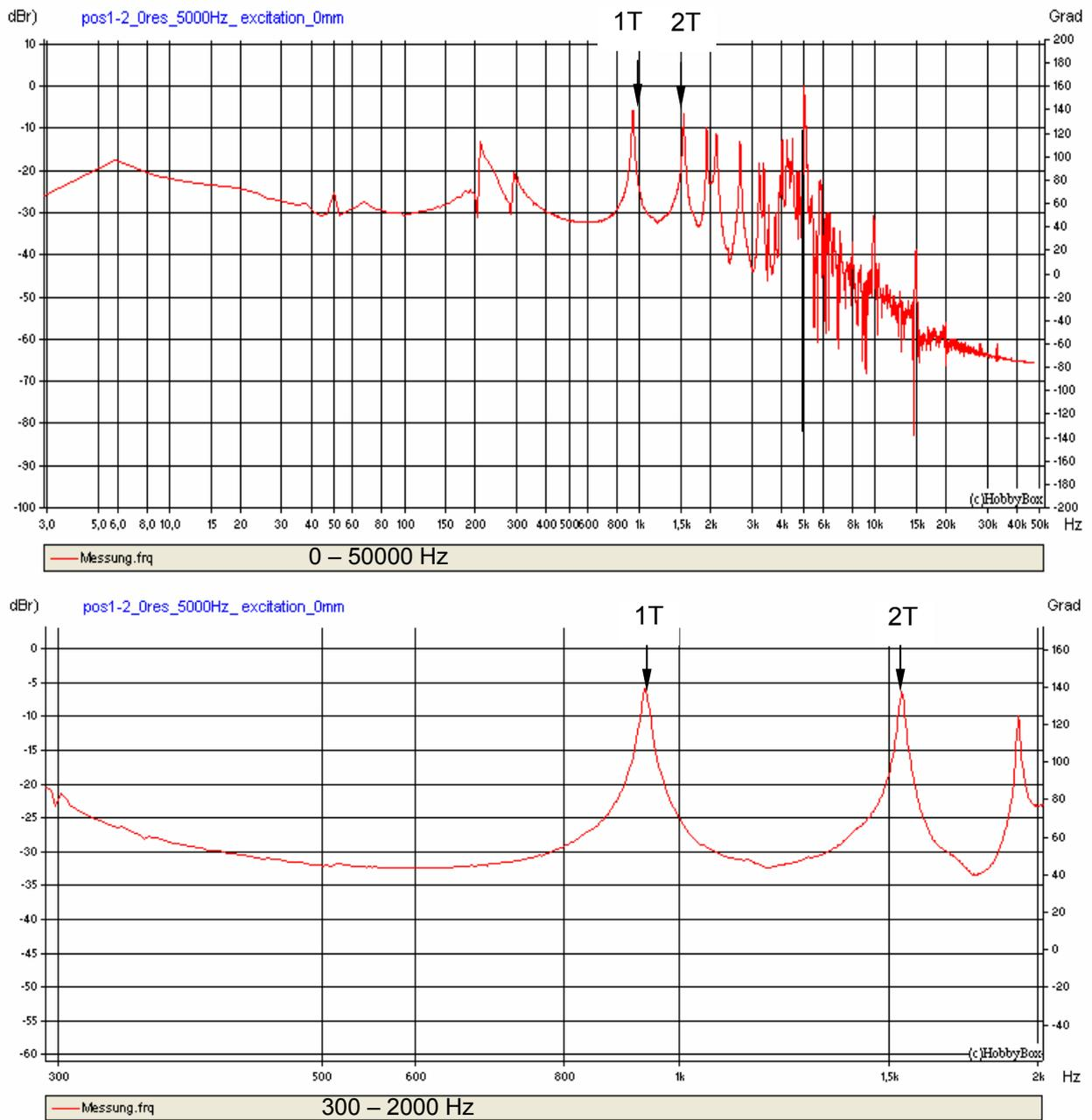
**Figure 3.4.1:** Frequency response, position 1-2, resonator length 0 mm, 5000 Hz excitation
