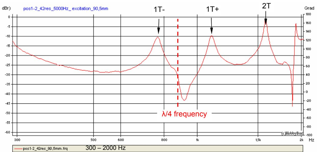
**Figure 3.4.3:** Frequency response, position 1-2, 42 resonators,  $L/R = 0,823$
