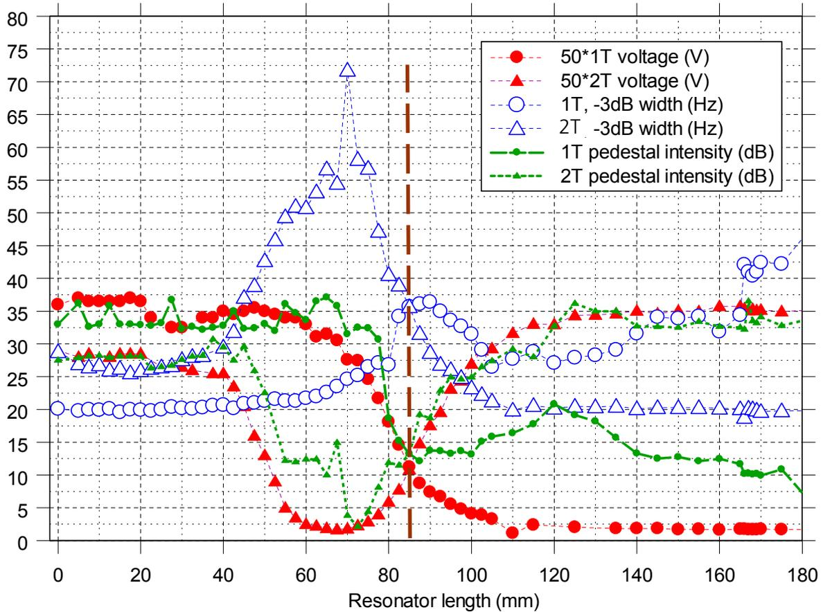
**Figure 1.6.1.:** Optimal length for damping 1T mode, CRC radius 100 mm [2]
