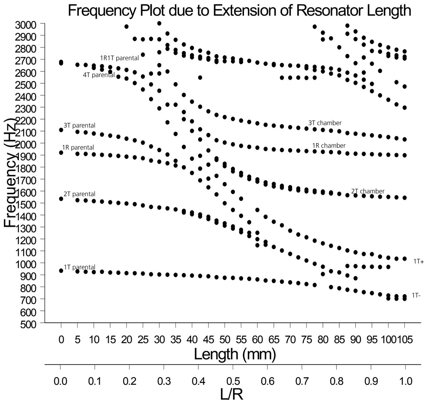
**Figure 3.3.4:** Measured course of the modes for position 1-2, 42 resonators
