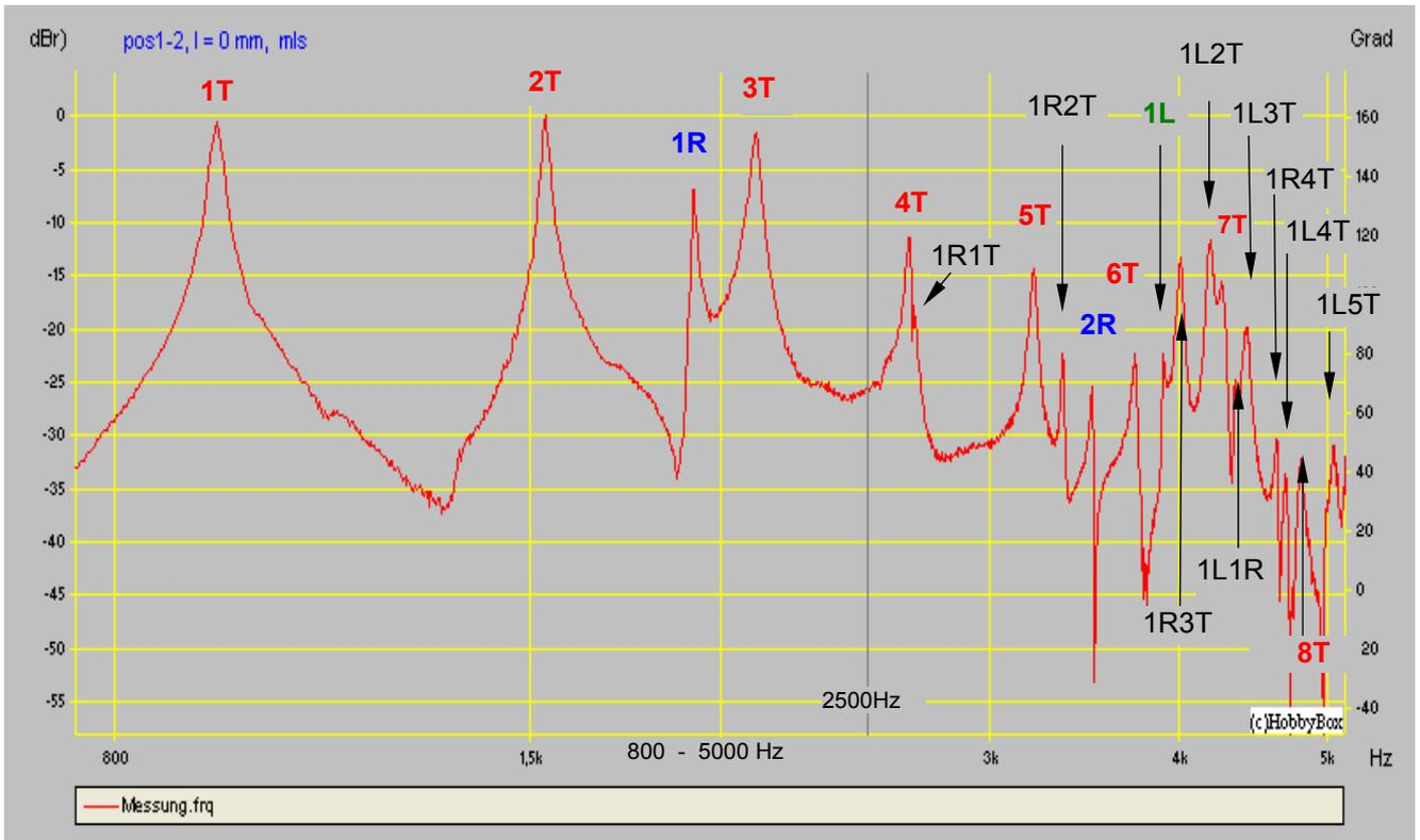
**Figure 3.3.1:** Overview of modes, position 1-2, resonator length 0 mm
