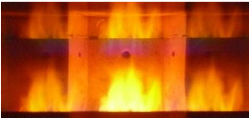
Bild 49: Glutphase,  $\lambda = 4,5$ ,  $\text{CO}_{13\% \text{O}_2} = 0,91\%$ ,  $\eta = 70 \%$
